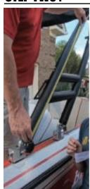
On the same **REAR** leg starting from the bottom move to the **OUTSIDE** of the leg and measure up 40" inches and mark center. Line this mark up with the **BOTTOM** hole of the swivel mount. Install screws. Place twist-knob in mount, head will face outward.
