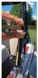
Starting at the bottom of the **REAR** tower leg, measure 17" inches up the **BACKSIDE** of the leg and mark center. Line this mark up with the **BOTTOM** hole of the strap eye. Install screws. Strap eye should run parallel with tower leg.
